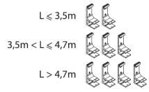
It is recommended to mount the outer wall brackets at a distance of 20 to 45 cm from the ends of the awning, and place the remaining brackets at equal intervals.
